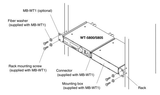
• When mounting two WT-5800/5805 units, use an optional mounting kit MB-WT2.
